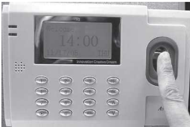
Figure 14.15 Biometric device (fingerprint)
