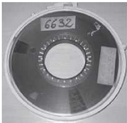
Figure 3.7 A 10.5-inch reel of 9-track tape
